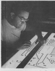
TOUCHING UP a duplicate master, a contact photographic print of the original drawing, is done by Bob Velasquez. He checks for defects and adds any necessary markings for the production of the
